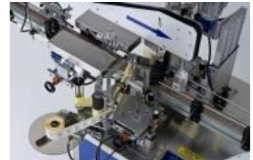
Realigning system and upper stabilization belt
