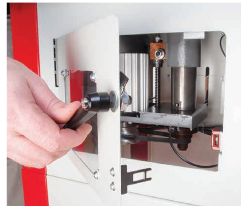
Motor and spindle access door
