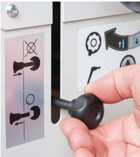
Turn the spindle & press in the locking knob to lock the spindle
